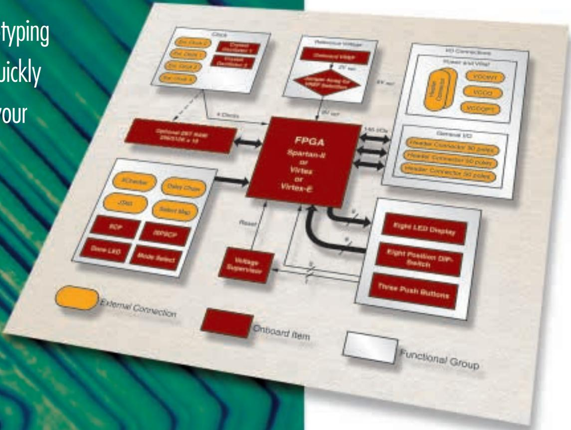
Figure 1 - Functional diagram of the development board modules
